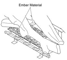
Figure 49 - Placing Ember Material on Burner
